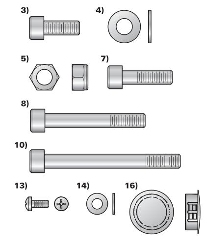
Attach the REAR SUPPORT (1) to the SEAT FRAME (2) using two M10 x 25mm BOLTS (3), four 3/8" SAE WASHERS (4), and two M10 NYLOCK NUTS (5) as shown. Tighten all BOLTS and NUTS securely.
